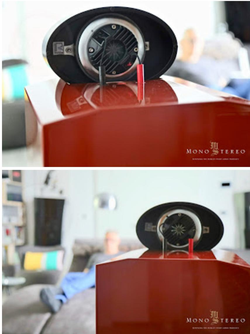
Another nice and highly useful feature is the selectable tweeter gain (1,5dB) as well as the tweeter's placement adjustment. The top plate of N° THREE enclosure lets you simply slide the tweeter forward and backward. This affects the time domain so that the broadband driver and tweeter can be time aligned if needed.
